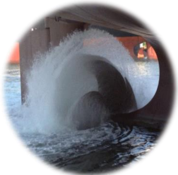
Propeller and Boss Cap Fins
